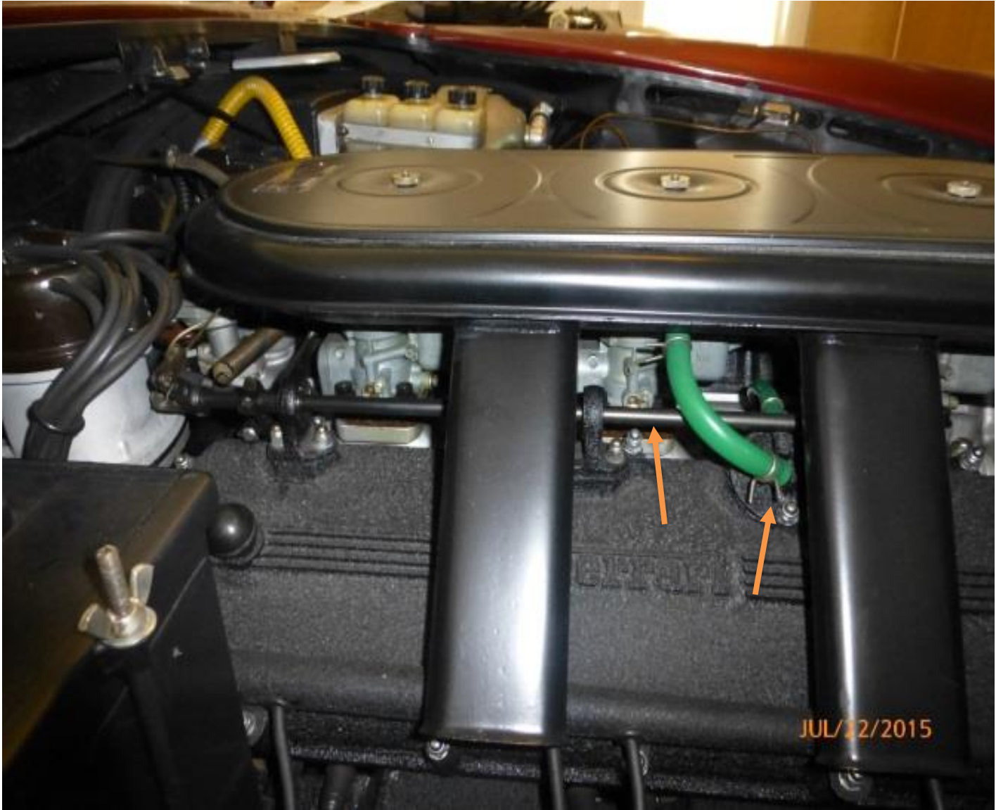
Throttle bell crank rod, black oxide Corbin spring clamp on breather hose
