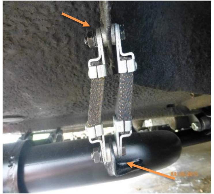
One spacer on each side of the exhaust brackets
