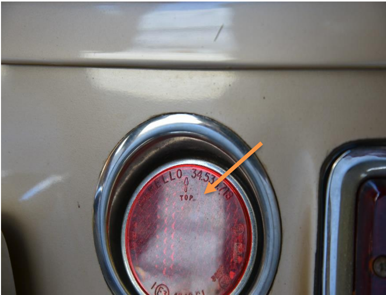
Carello reflector lens, TOP, or ALTO at the top of lens
