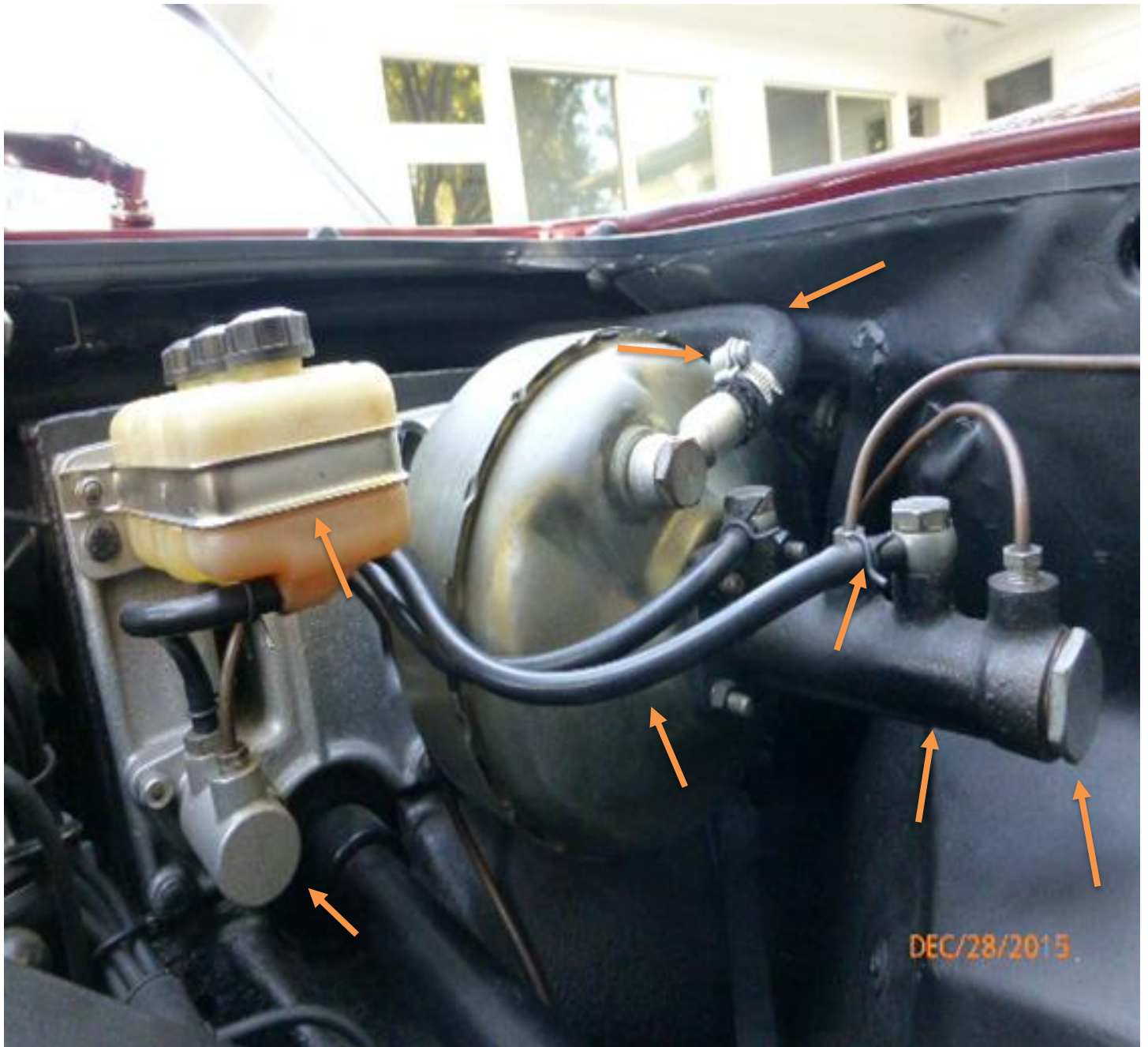
Bonaldi brake and clutch system
