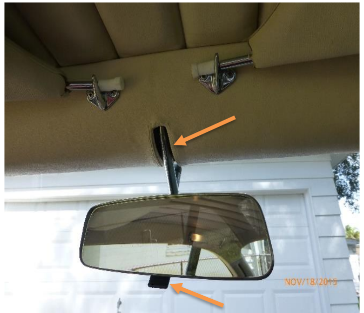
The mirror was mounted thru a slit in the fabric. Mirror had a lever to flip from day to night driving.
