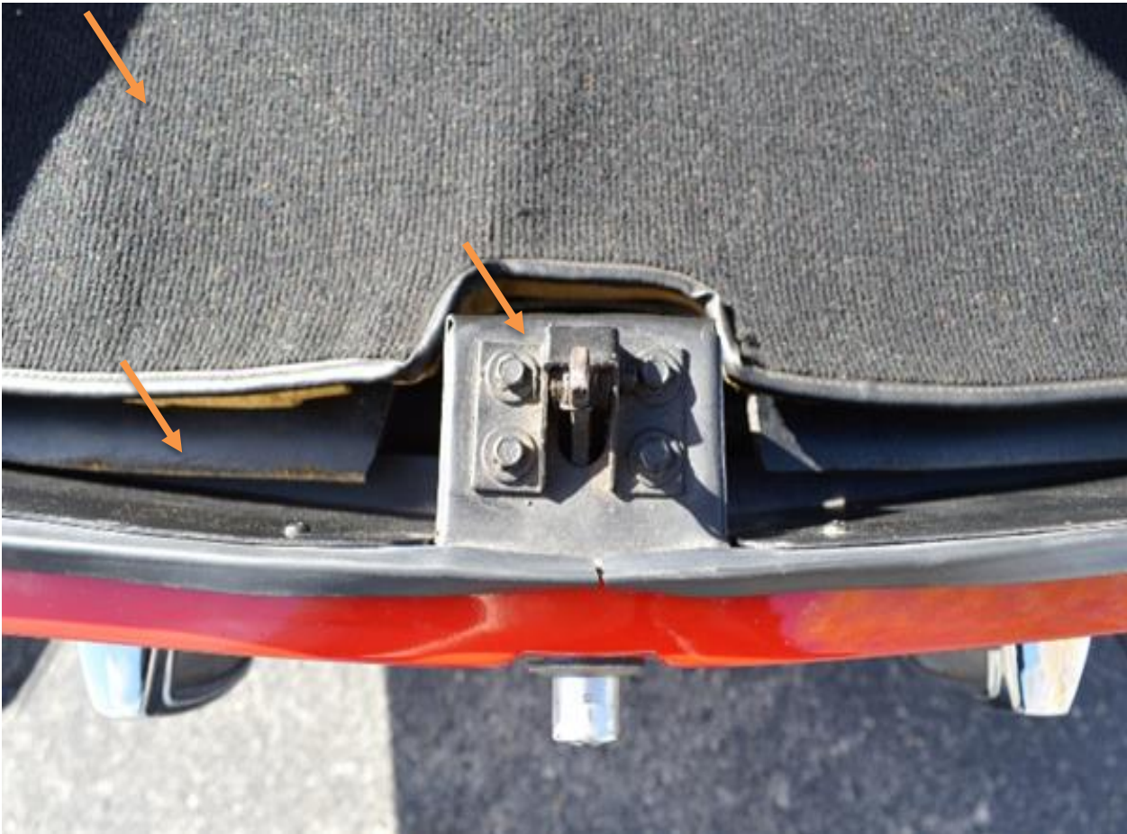
Masonite board covering spare, trunk latch does not have a cover, carpet same as 330 GTC
