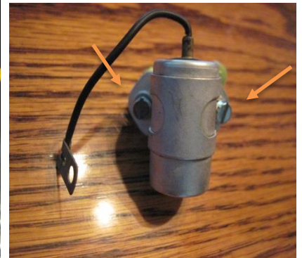
Capacitor has 2 mounting screws
