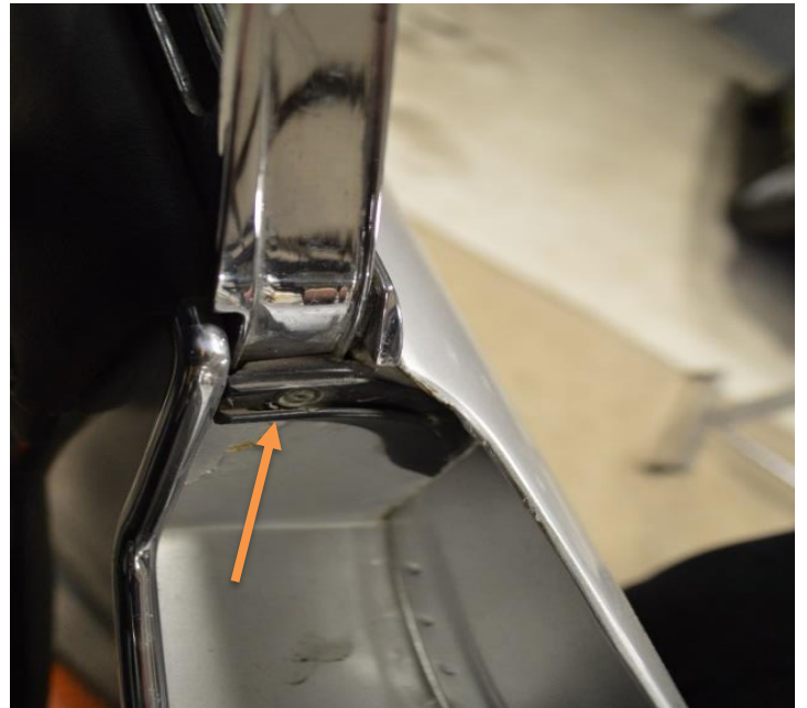
Unrestored car, molded rubber pieces where the front and rear window frame meets the door.
