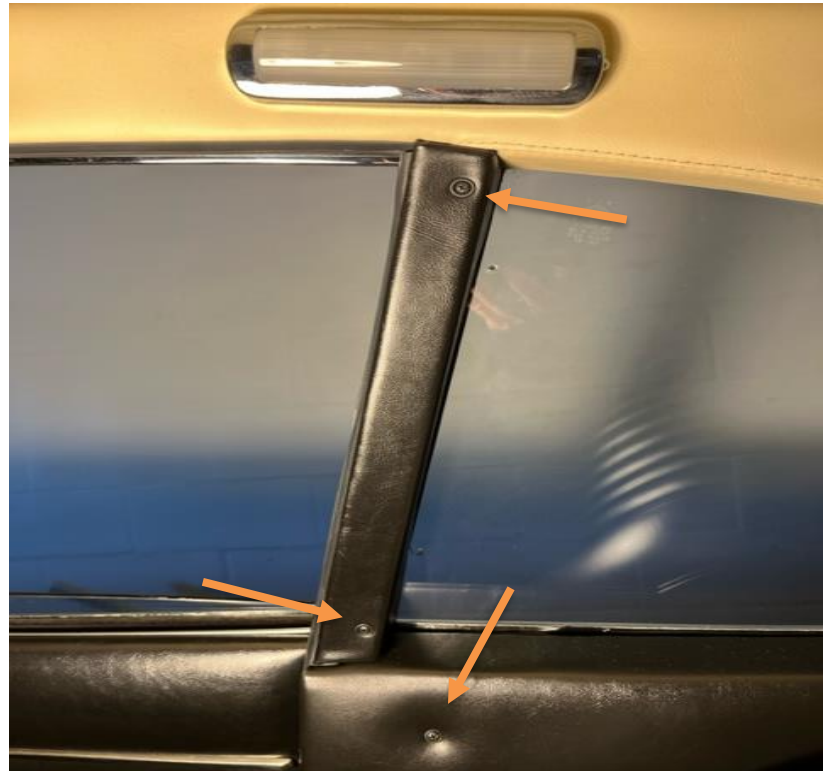
Black oxide Phillips head screws and cup trim washers
