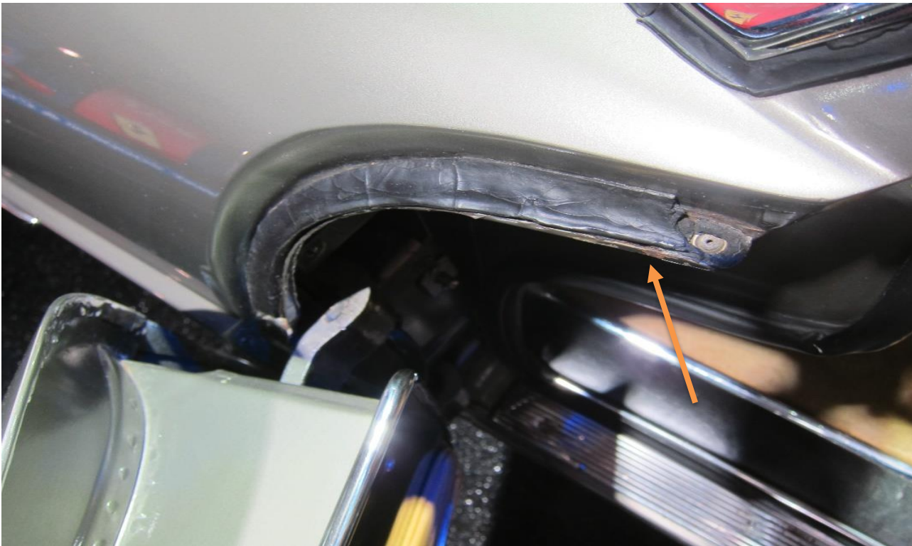
Unrestored car showing rubber weather seal and pop rivet
