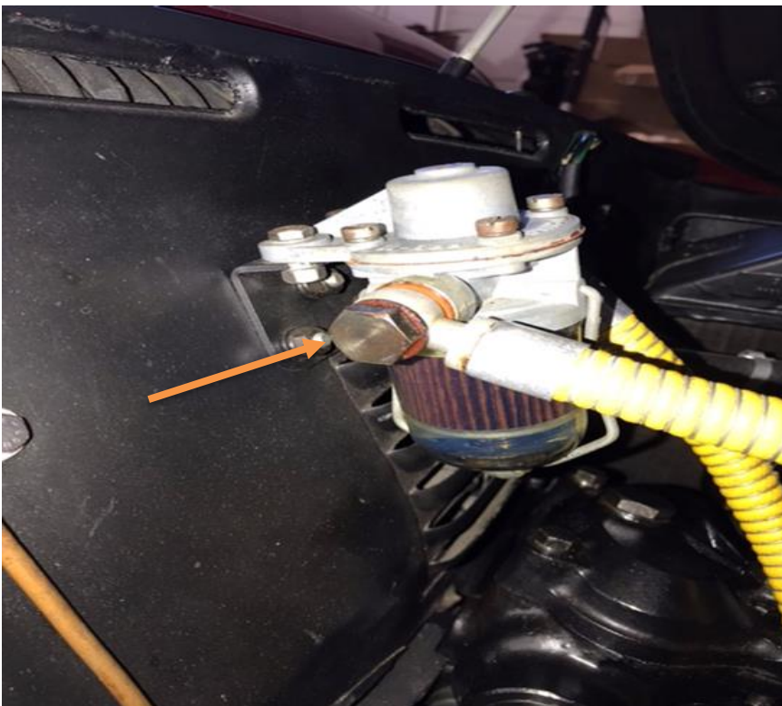
Black Oxide banjo bolt securing fuel line
