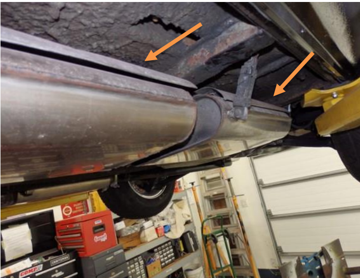
Heat shield over mufflers
