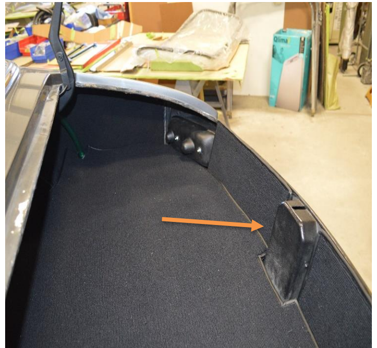
Molded trunk latch cover with angled top
