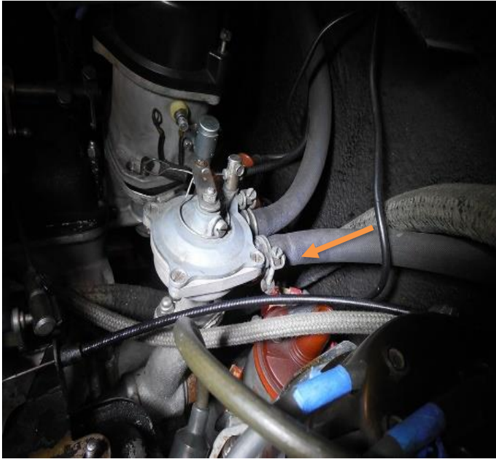
Angst clamp on heater control valve #10767
