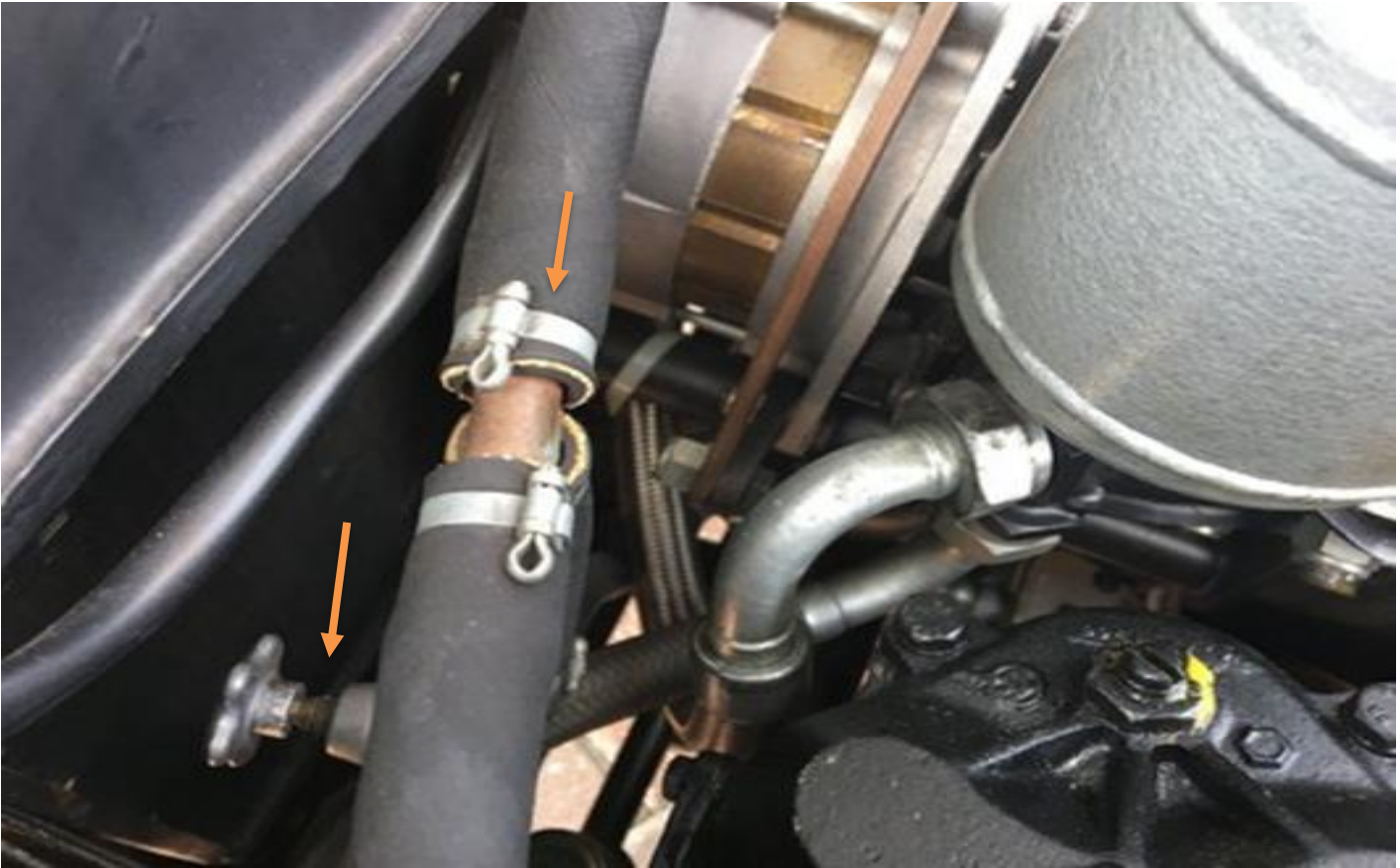
5mm Copiglia clamps on cloth wrapped heater hose and heater valve cutoff below the T junction
