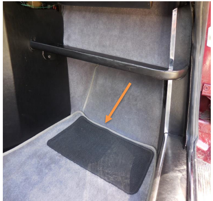
Passenger heel mat not on firewall
