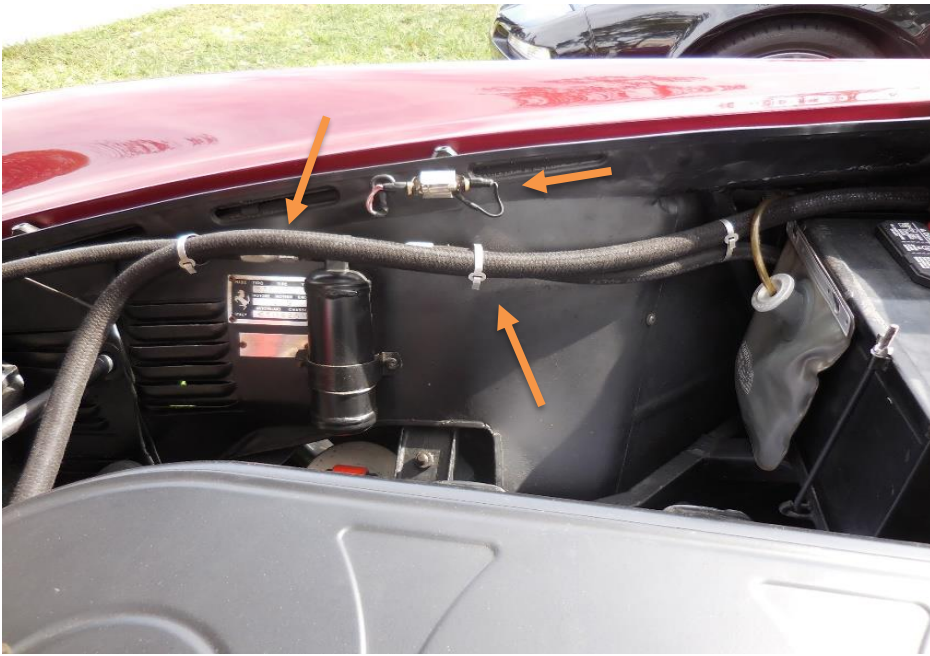
AC hoses, dryer, engine bay light, metal ties on hoses
