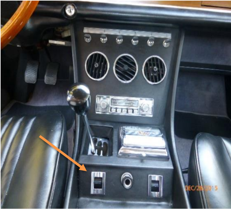
Window switches are made by Ducellier.
