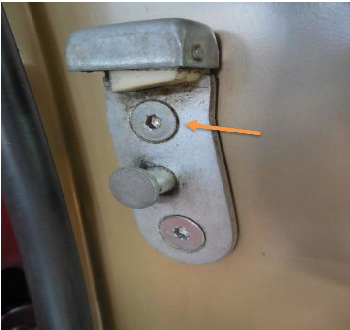
Unrestored car door striker mounting, allen head screws
