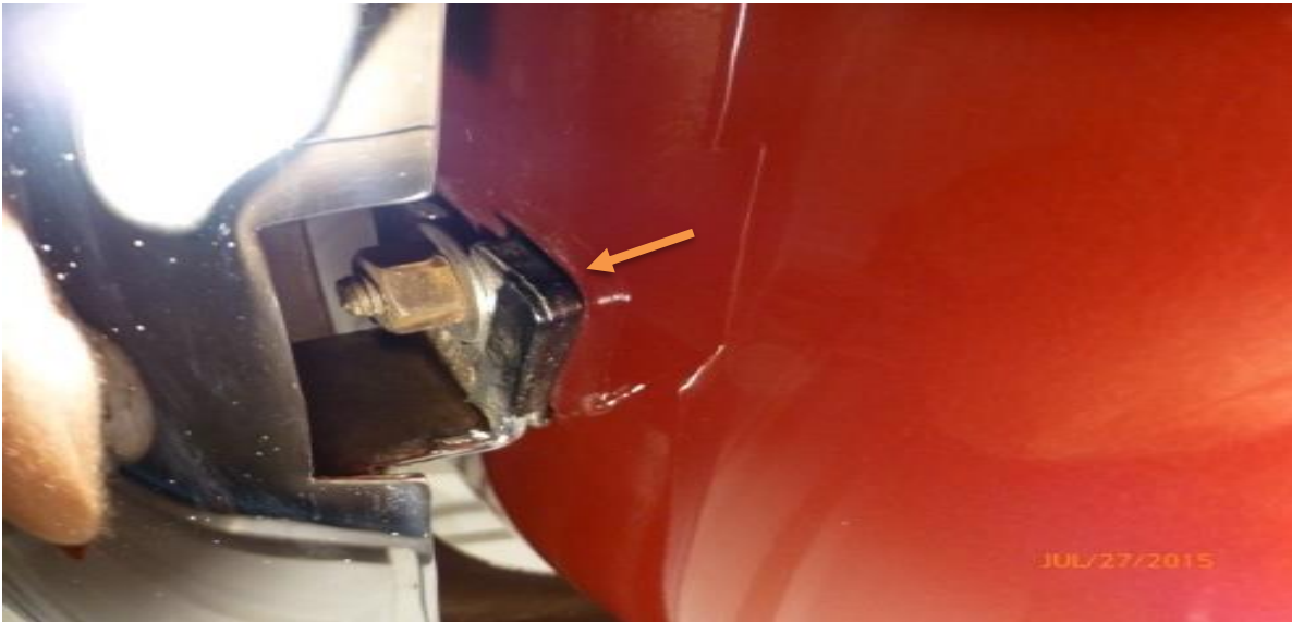
Location of spacer between rear bumper and fender
