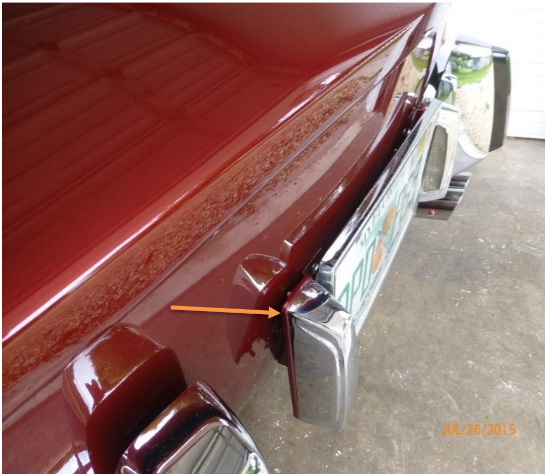
Bracket behind license plate lights painted body color
