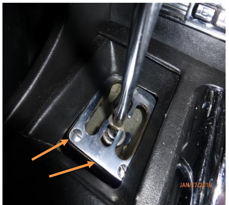
Shift gate plate with slotted screws
