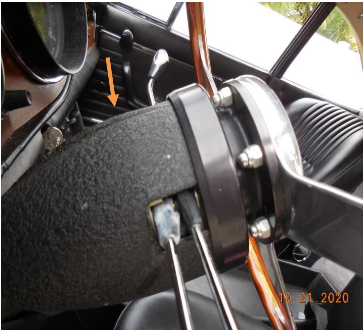
Steering wheel mounted with 6 mm acorn nuts, wrinkle finish
