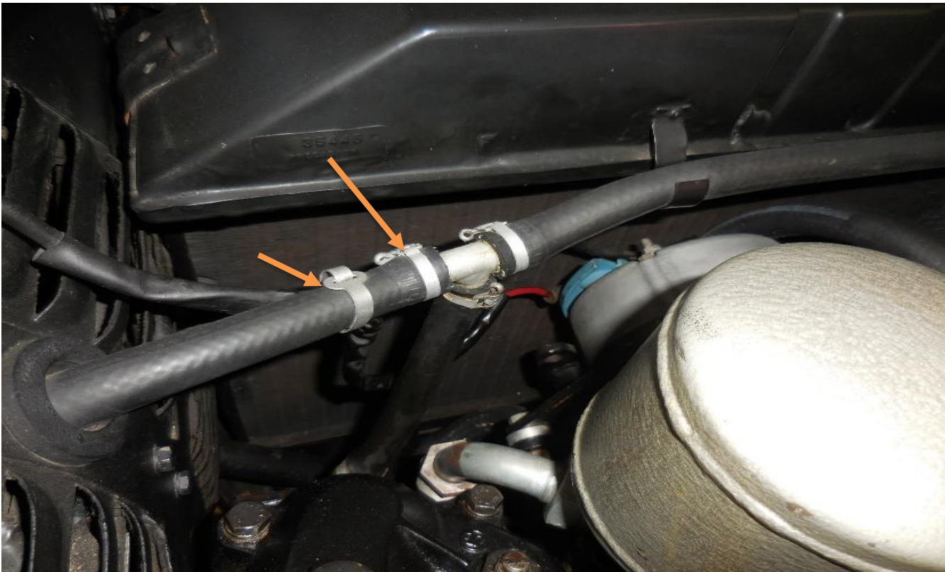
Copiglia clamps on water hoses and metal tie on alternator wires
