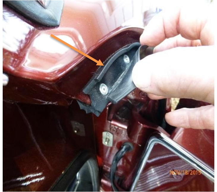
3/32 pop rivets and flat washer
