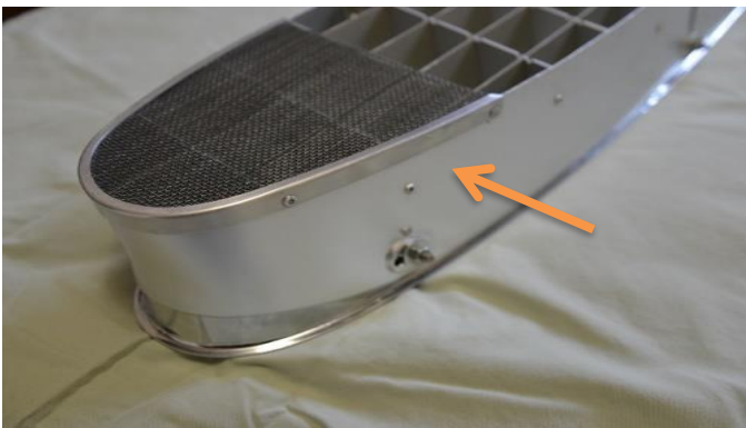
Method for mounting the wire screens
