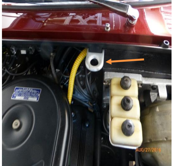
Later production car hood latch bracket with round hole in the middle
