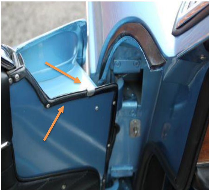
Early cars had a rubber molding and metal clip
