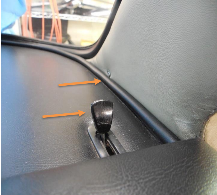
Fuel door opening lever with fan shaped knob and welting
