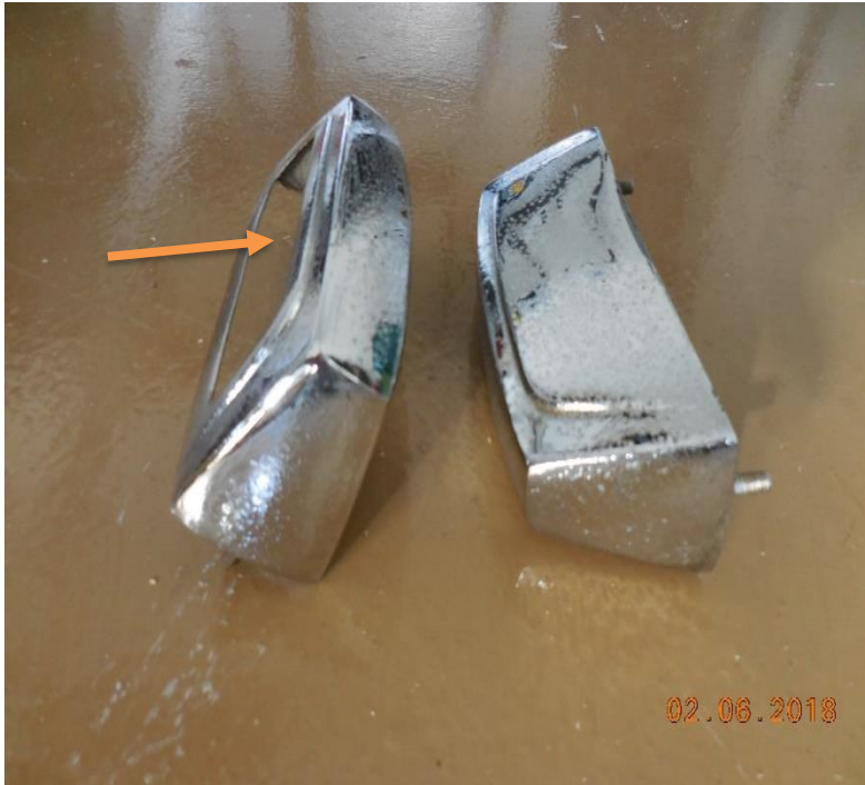
Unrestored license plate light fixtures showing the very small lip on the lens side and raised area on the back side
