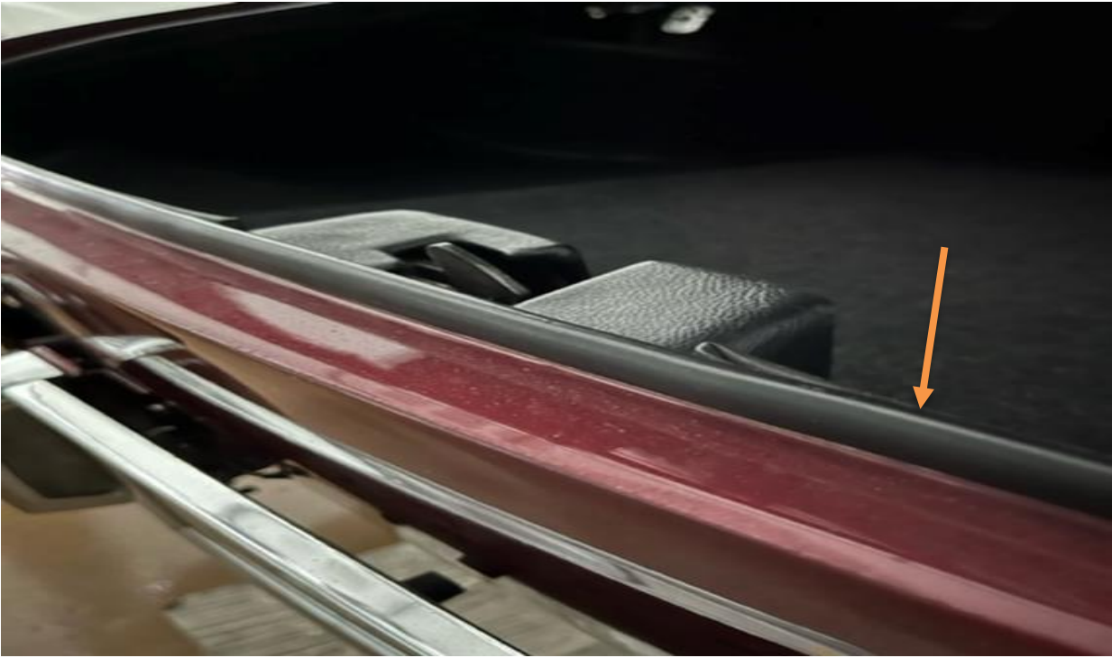
U shaped rubber molding covering trunk pinch weld.
