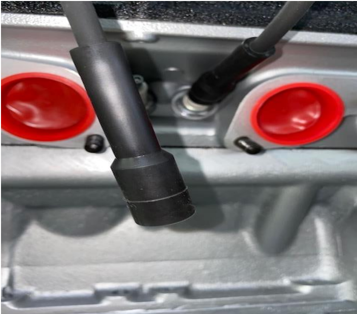
Spark plug wire rubber boot termination
