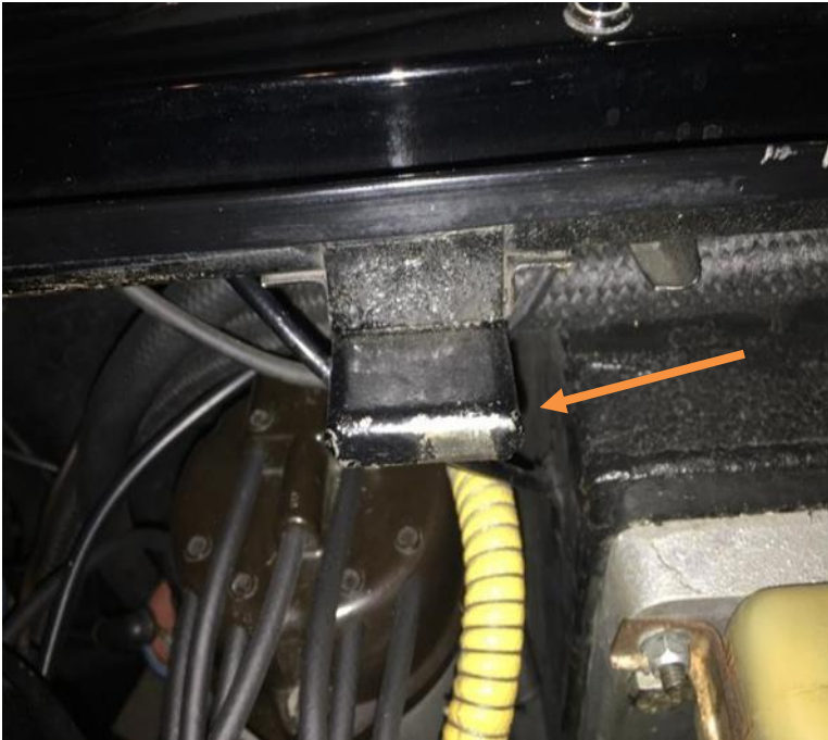
Early production car (8833) with flat hood latch bracket
