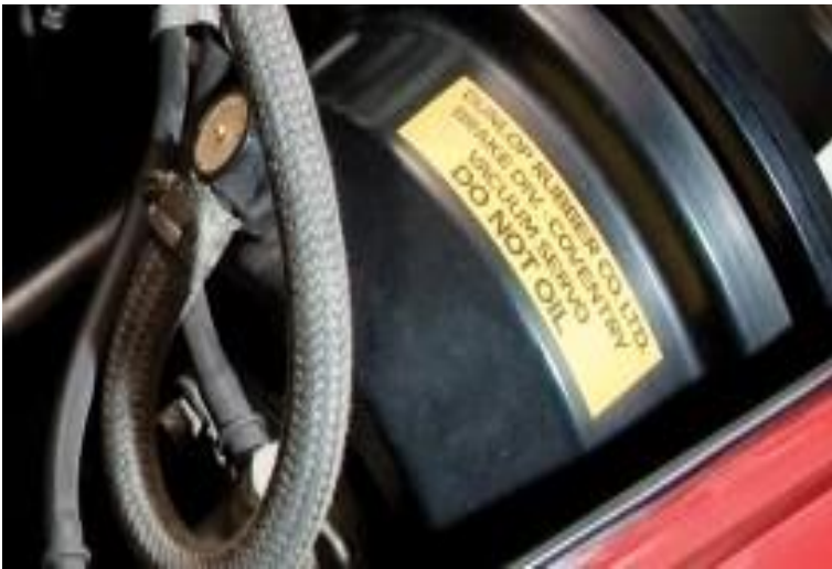
Do Not Oil label on Dunlop brake servo
