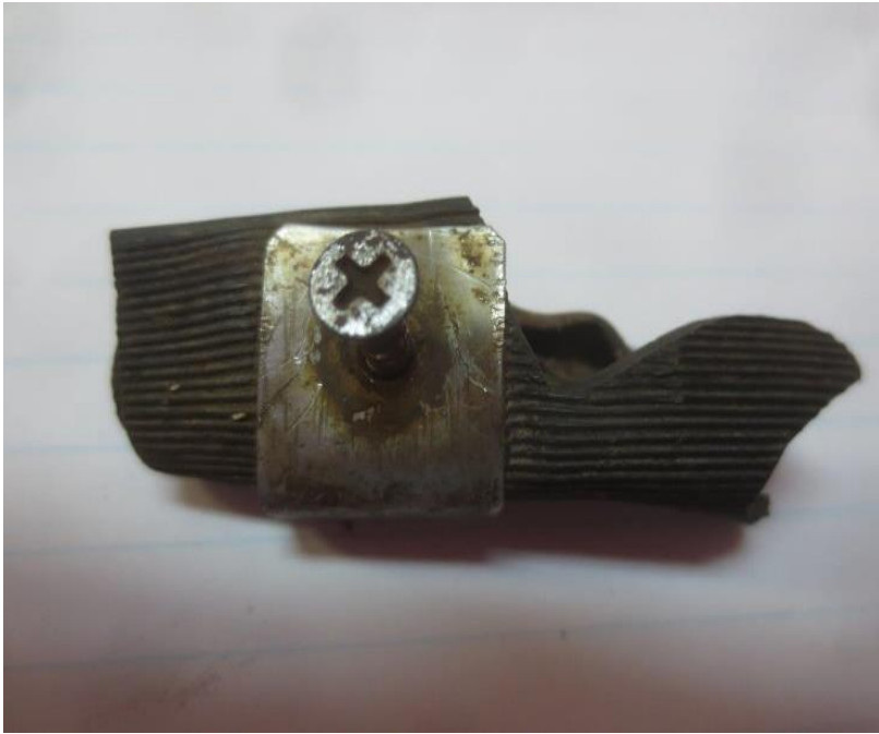
From unrestored car showing flat head Phillips screw, ribbed rubber molding and chamfered corners S/N 9959
