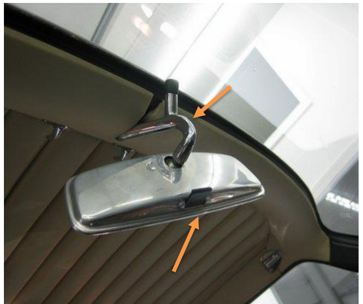
Mirror mounting bracket is chrome Mirror back side is polished aluminum
