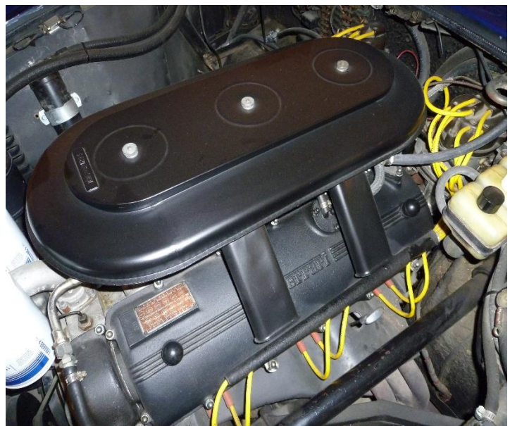
Air filter on S/N 9605 (yellow plug wires are not correct)
