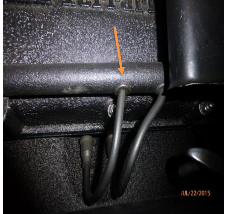
Rubber grommets protecting plug wires
