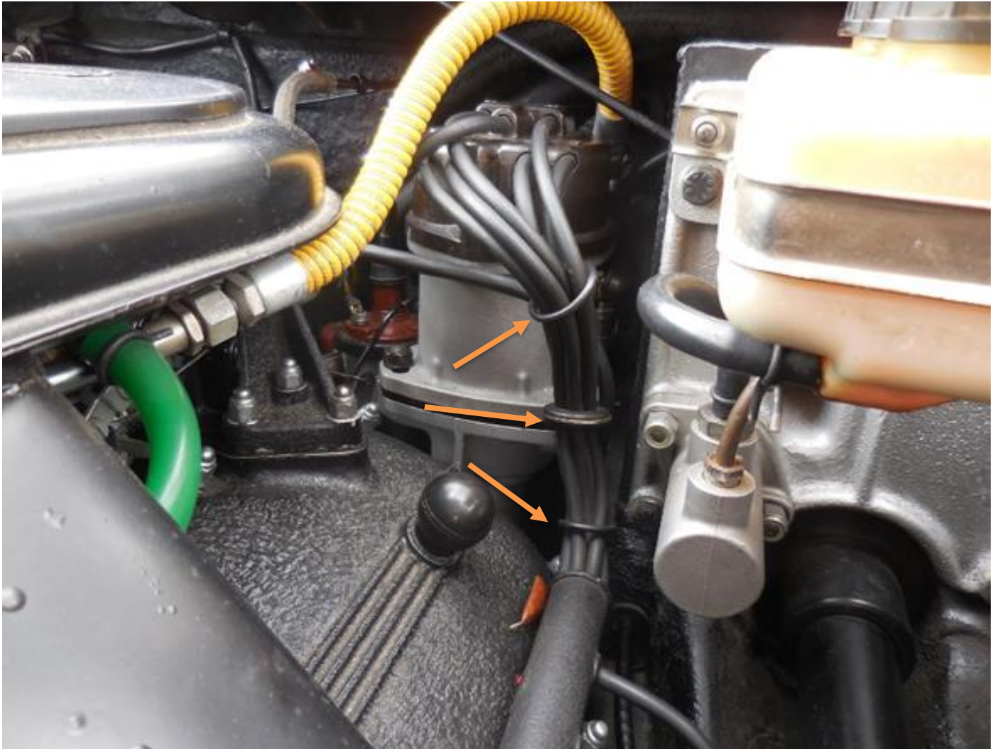
Retaining bracket on distributor and two O-rings gathering black 7mm plug wires, left side
