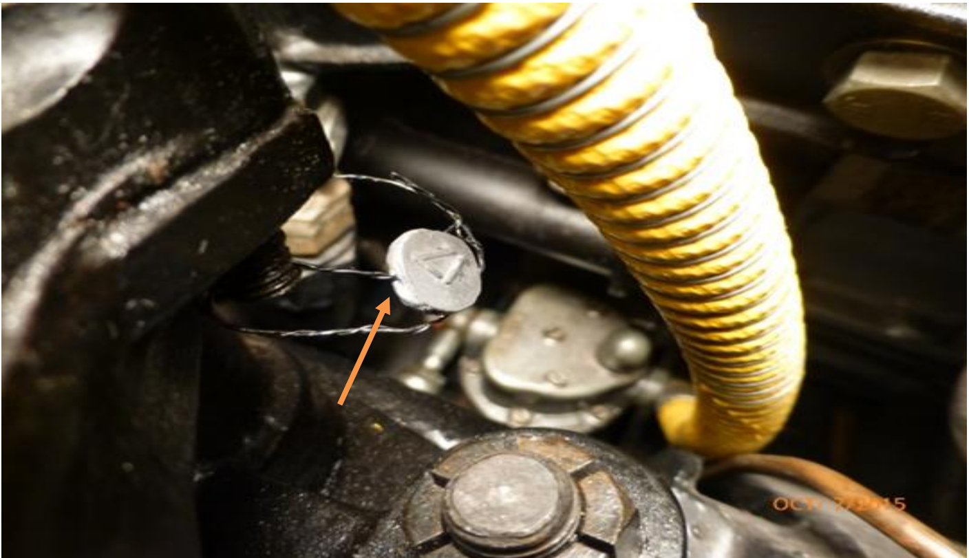
ZF lead tag on steering box
