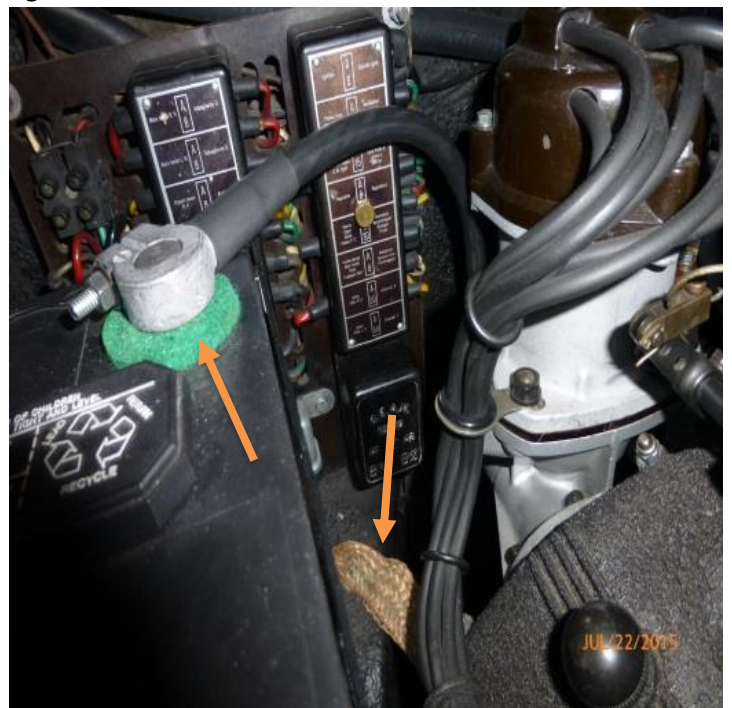
Negative terminal, copper ground strap
