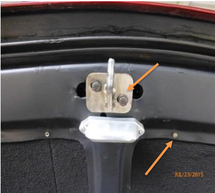
Brass nuts holding Ferrari and 330 scripts on trunk
