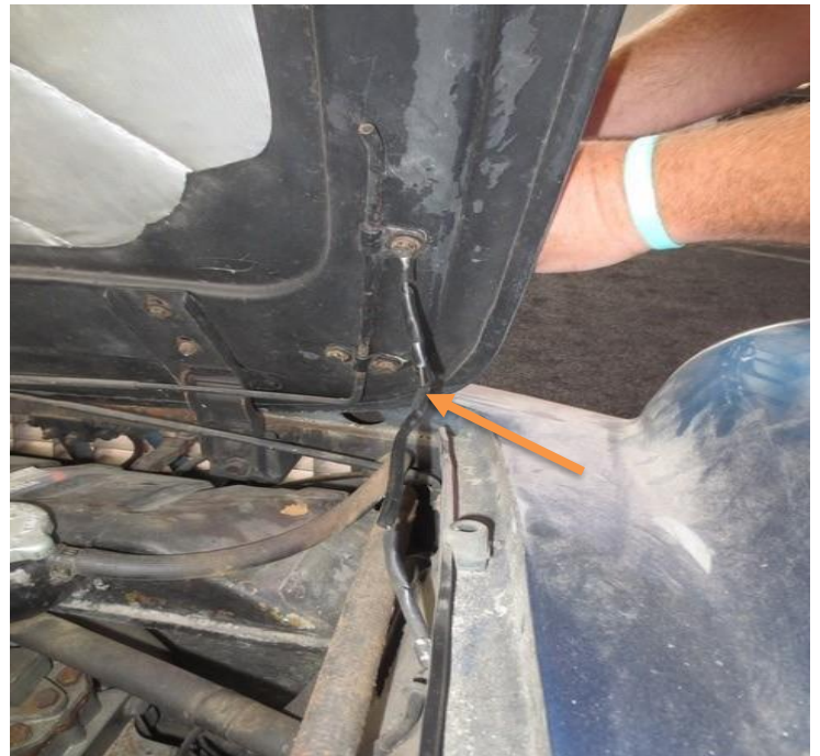
Hood retaining lanyard cable, unrestored car S/N 9605
