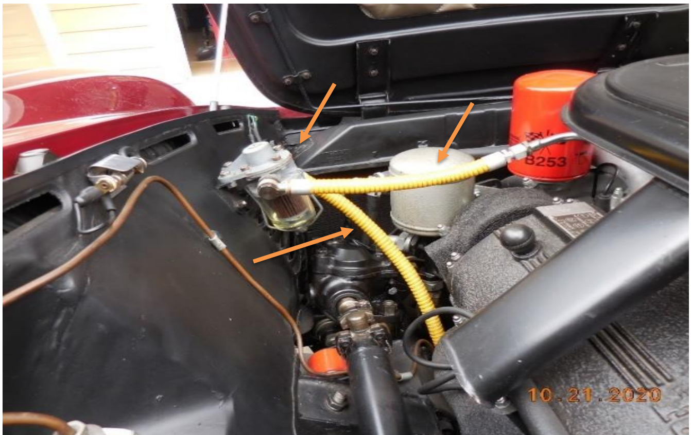
FISPA filter and yellow fuel lines
