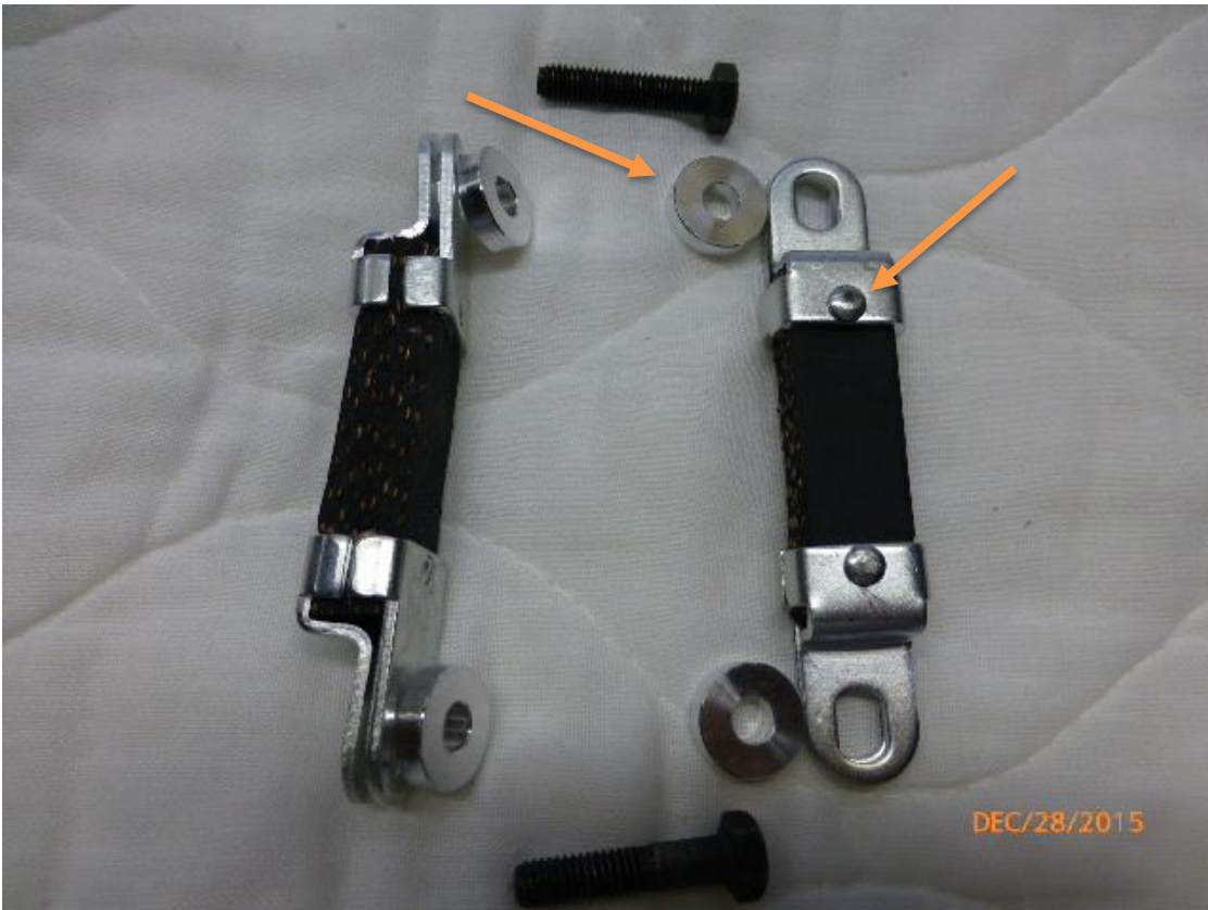
Solid riveted exhaust hanger straps and aluminum spacers
