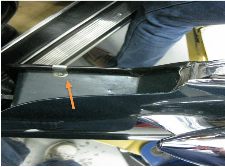
Clip on top of door to hold rubber trim
