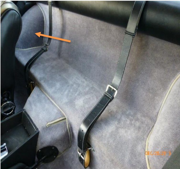
Carpet covering on inside wheelwell
