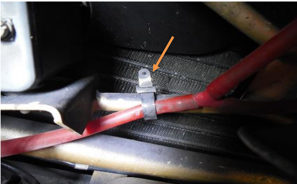
Unrestored car showing air horn tie S/N10767
