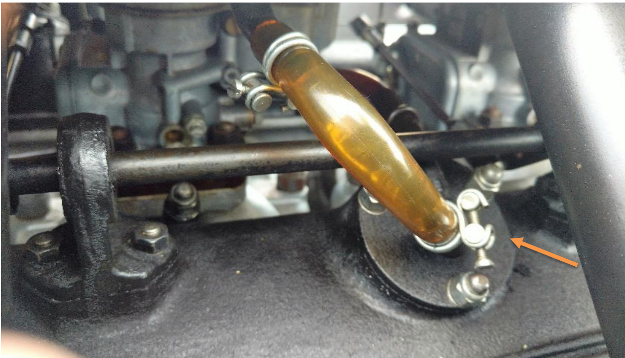
A later production car with Angst clamps on breather hose
