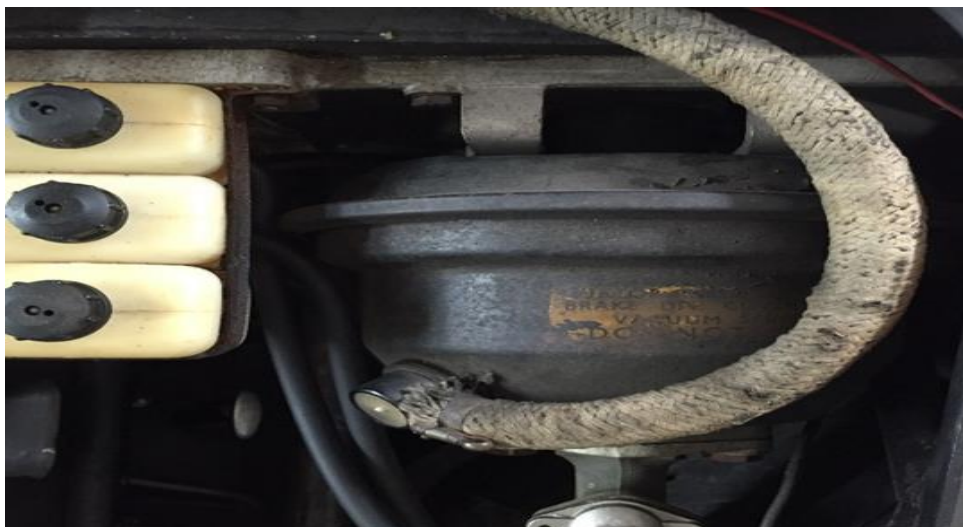
Unrestored Dunlop brake booster with Do Not Oil decal and Copiglia clamp on vacuum hose
