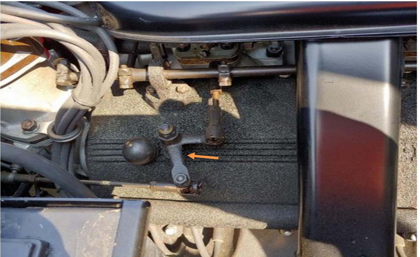
Bell crank rod drive mechanism on right side valve cover on later production cars 11271
