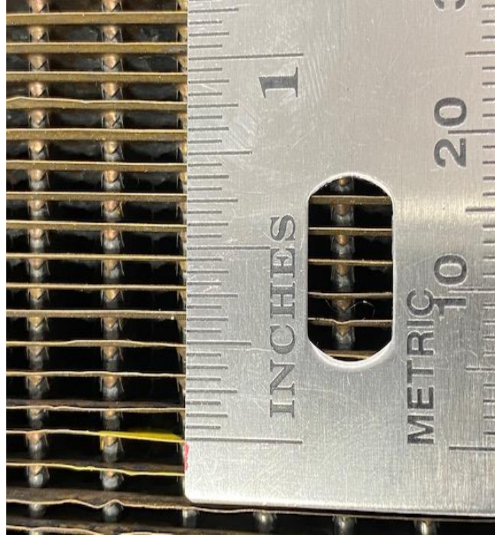
Original radiator with continuous horizontal fins
