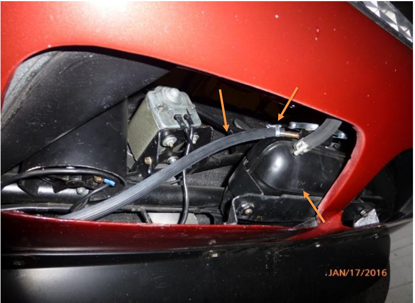
Radiator overflow tank , ribbed hose, Copiglia clamps
