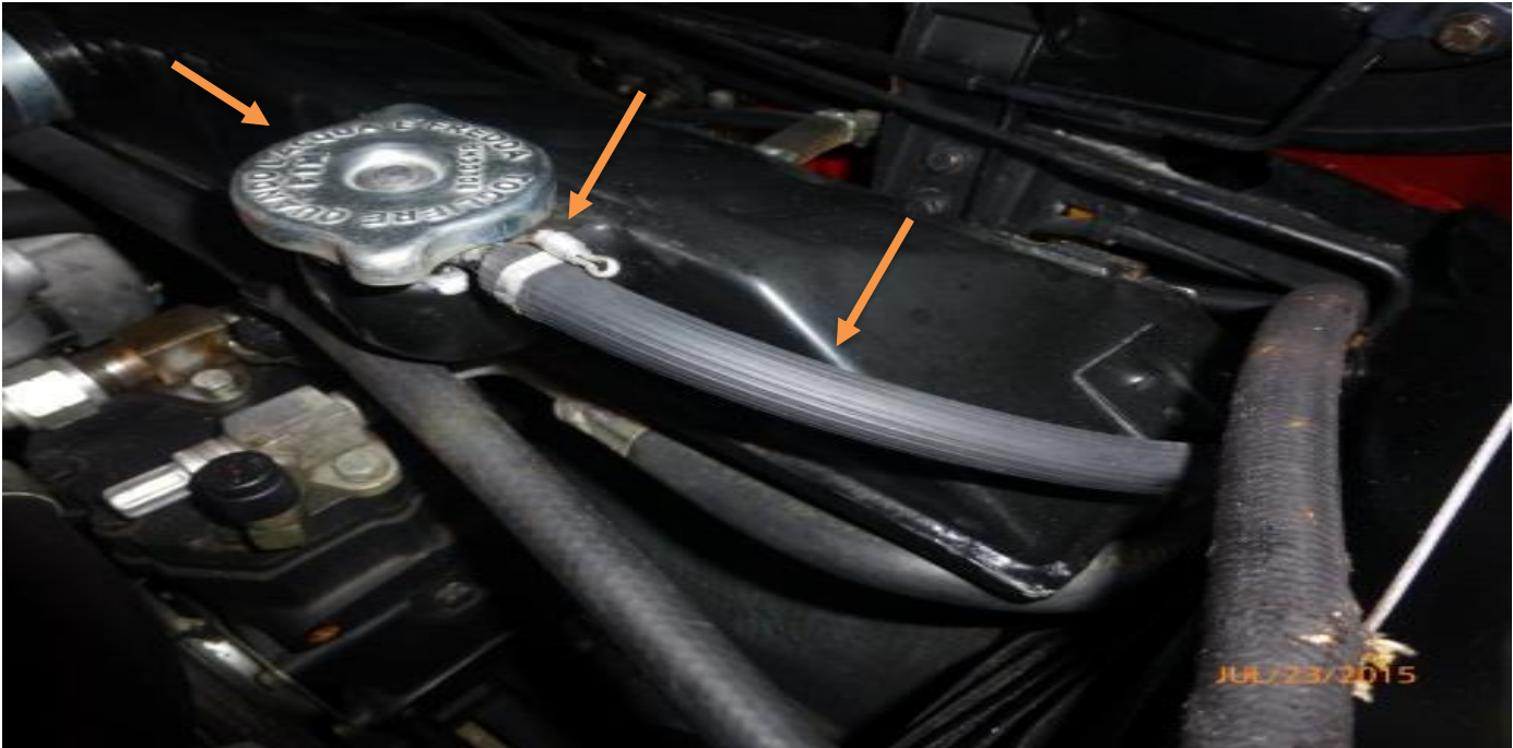
Non pressure radiator cap, ribbed overflow hose and 5 mm Copiglia clamp
