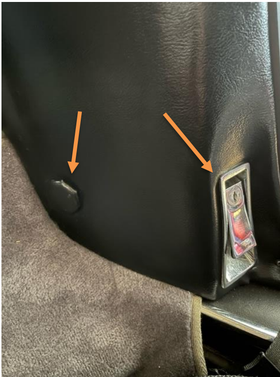
Trunk pull lever and emergency cable access
