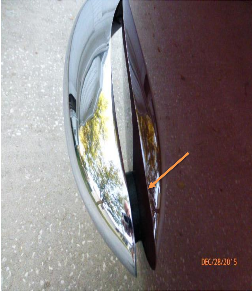
Rubber spacer between bumper and fender
