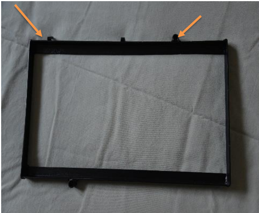
Battery hold down bracket, and hooks
