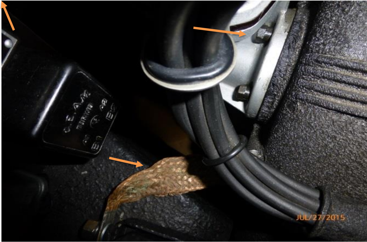
Special 4mm bolts mounting the distributor to the valve cover, copper strap
