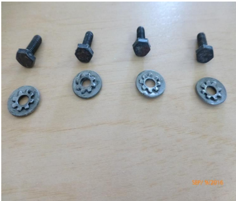
Bolts and washers to mount fuel filler tube hex bolts, star, and flat washers.
