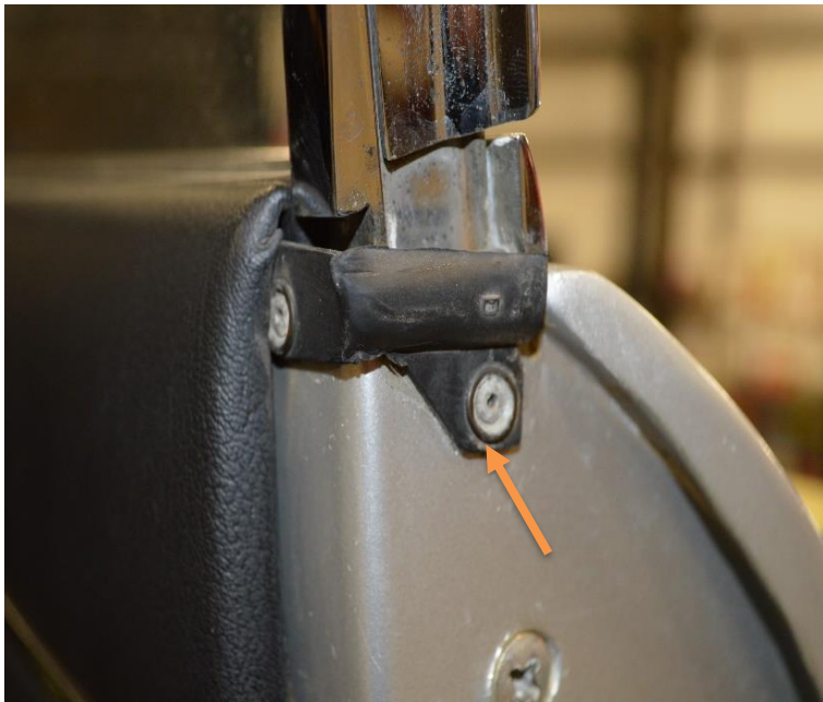
Unrestored car, molded rubber pieces where the front and rear window frame meets the door.
