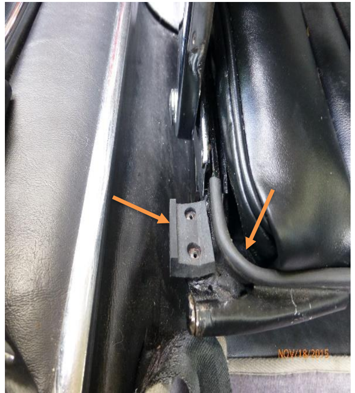
Seat back rest stop rubber molding on edge of seat bottom
