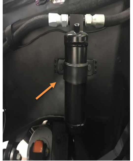
Dryer support bracket mounted with pop rivets 8843
