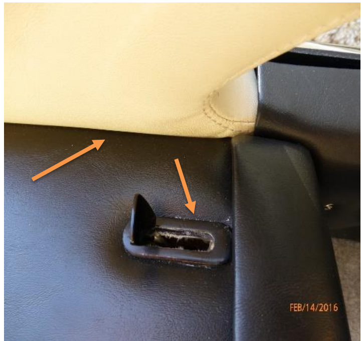
Black satin bezel around lever shaft (welting is missing)
