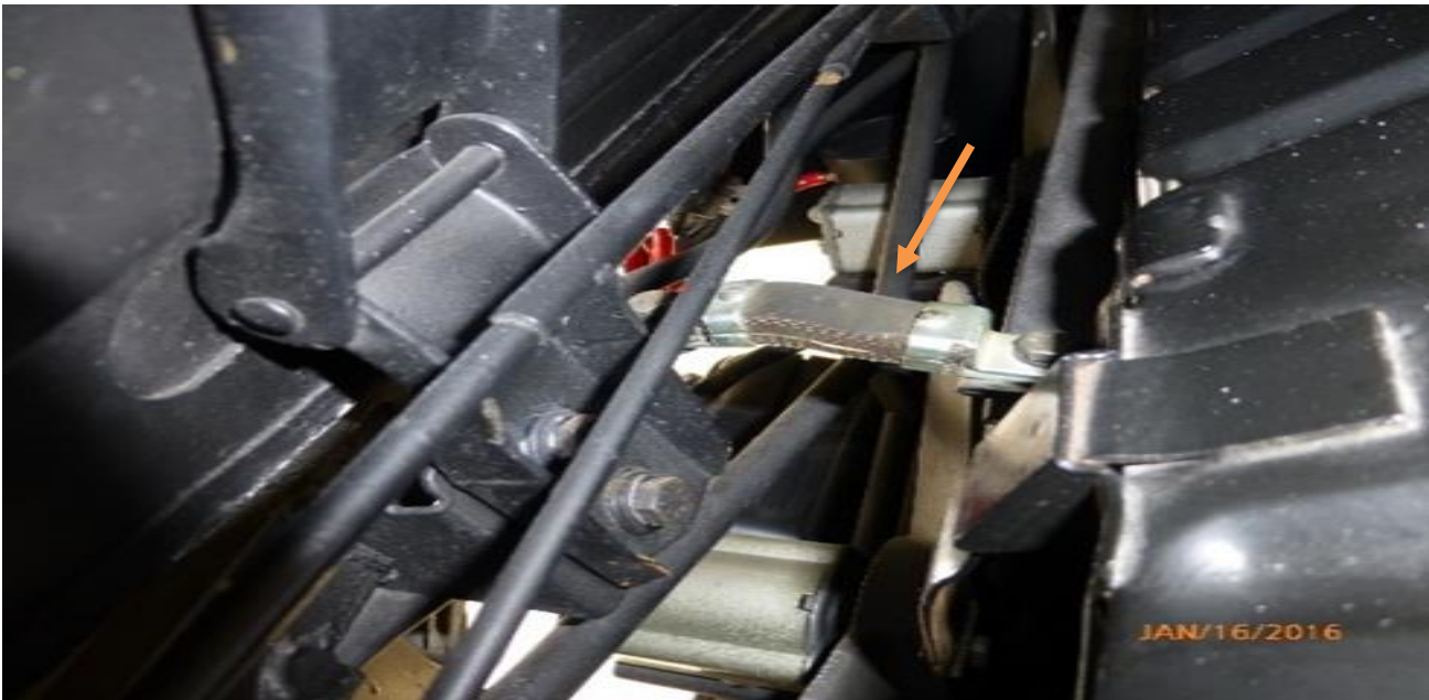
Strap between radiator and chassis
