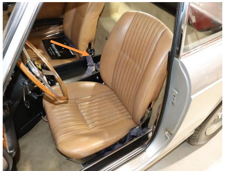
Back rake adjustment on center console side
