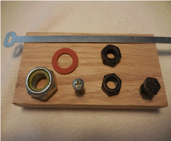
Nuts, Phillips head screw, metal tie, red fiber washer, Lobo bolt
