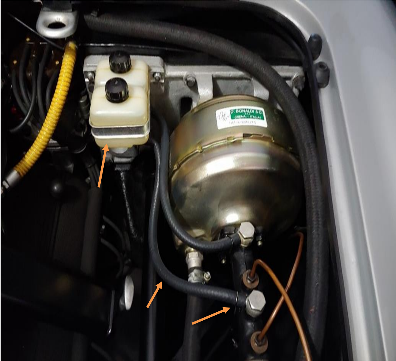
Late production car with mechanical clutch, only 2 brake fluid reservoirs S/N 11271, smooth hoses, Corbin spring clamps
