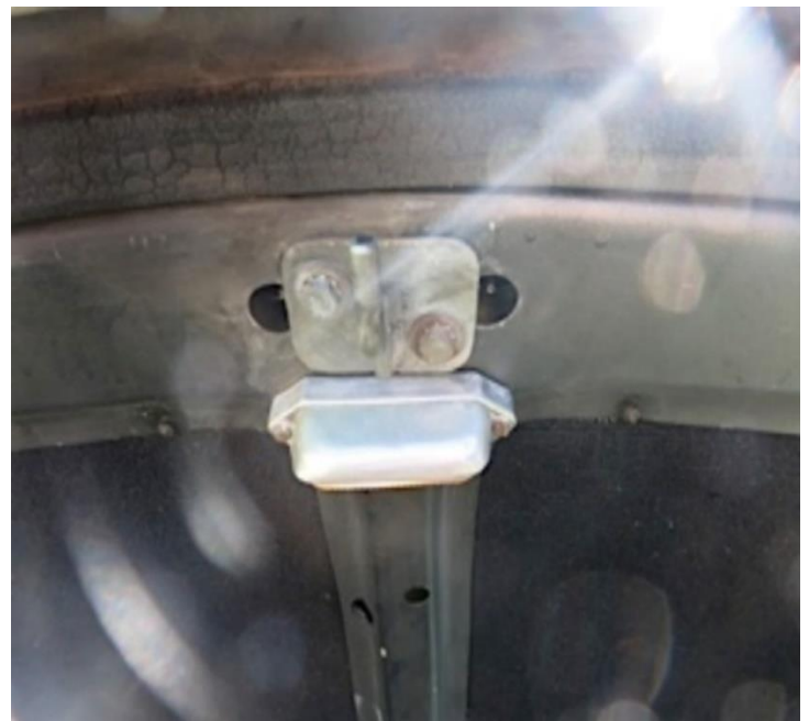
Unrestored car trunk latch with silver CAD Lobo bolts
