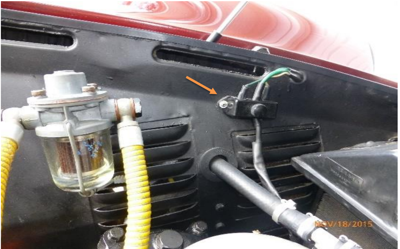
Junction box for alternator wiring connection
