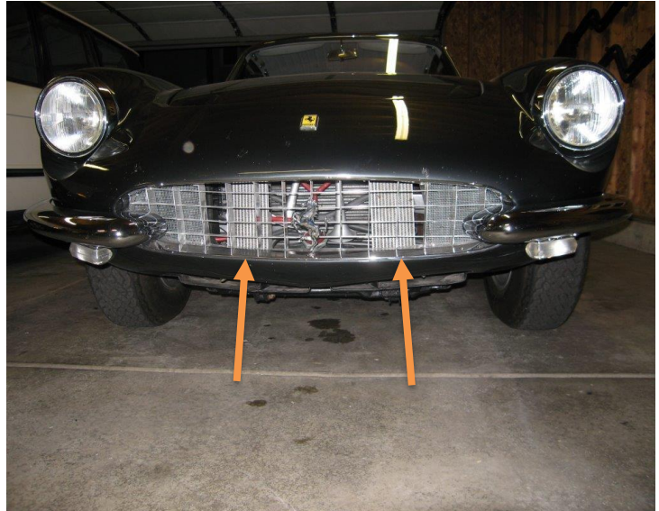
Restored car showing 2 oil coolers
