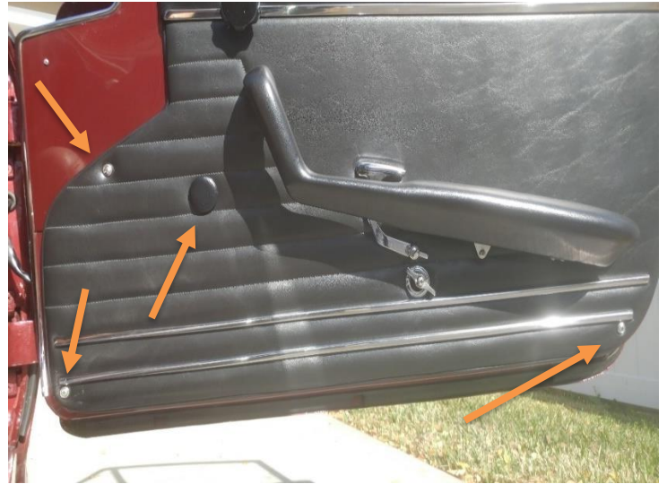
Emergency window crank access hole, three door panel screws
