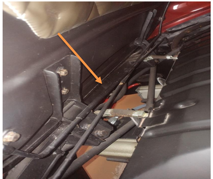
Hood spring rods and rubber tube over the rod
