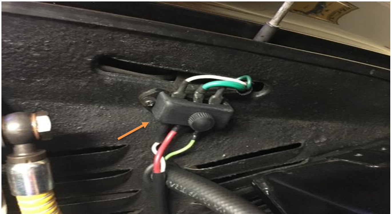
Junction box for alternator wiring connection
