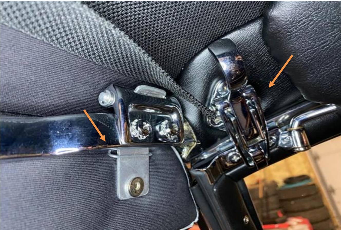
Top latching mechanism and side flap
