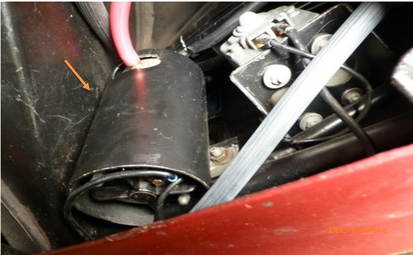
Fiamm air horn compressor inside plastic can
