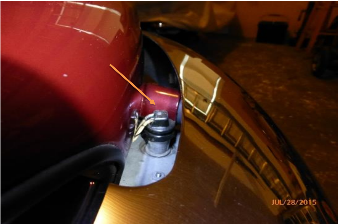
Rubber boot over turn signal/ running light fixture
