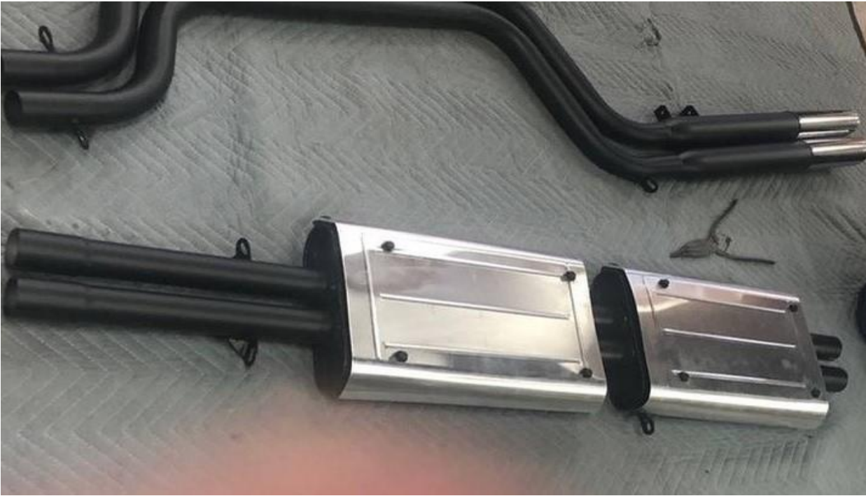
Heat shield over mufflers
