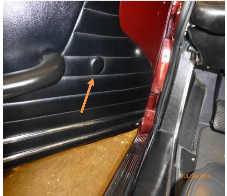
Access hole in door panel for emergency crank
