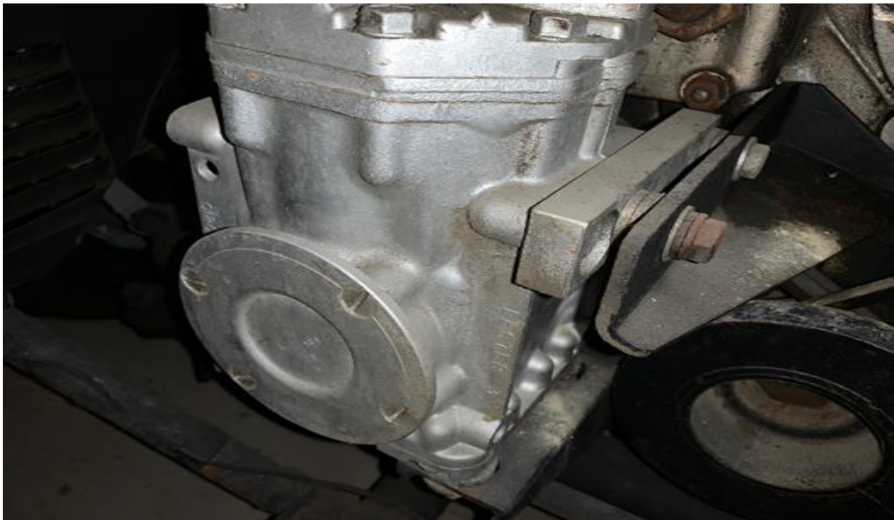
AC Compressor in unrestored car S/N 9605
