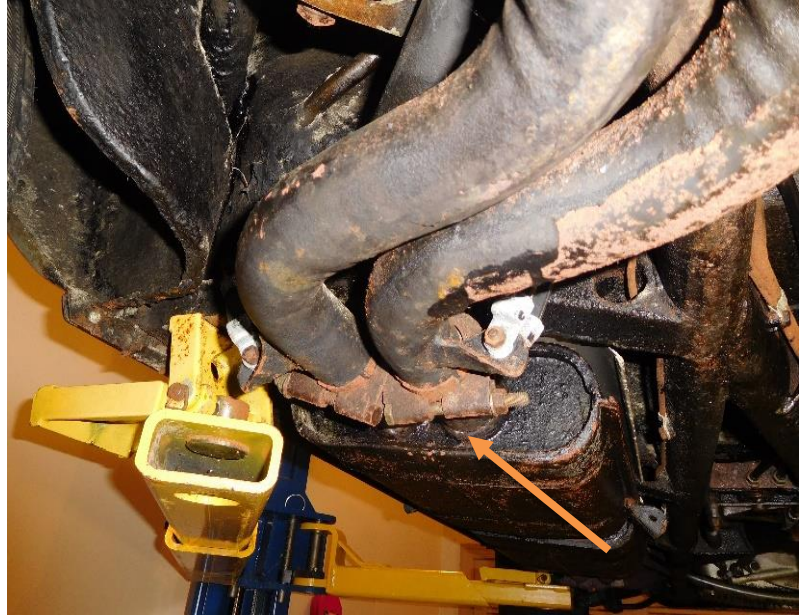
Exhaust clamps on unrestored car
