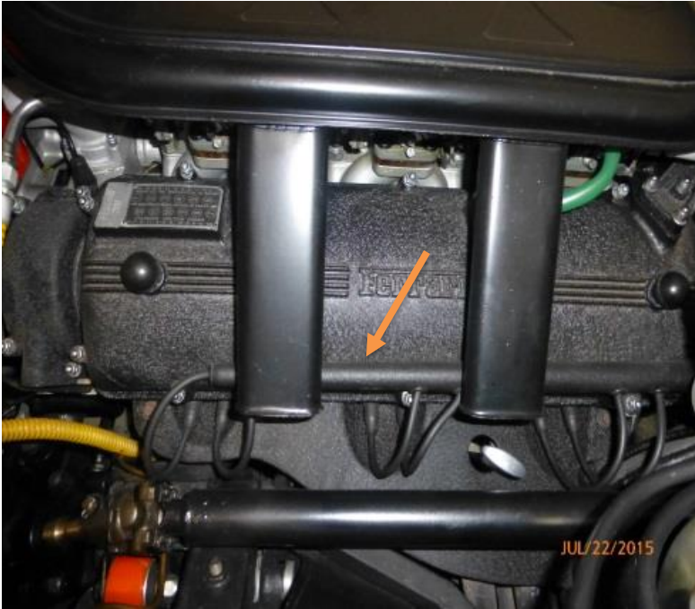
Tapered metal distribution tube for plug wires
