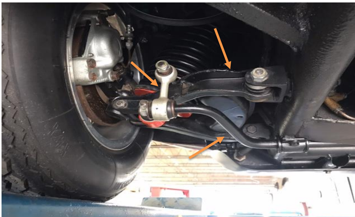
Front suspension black satin A arms and sway bar, dull nickel dog bone
