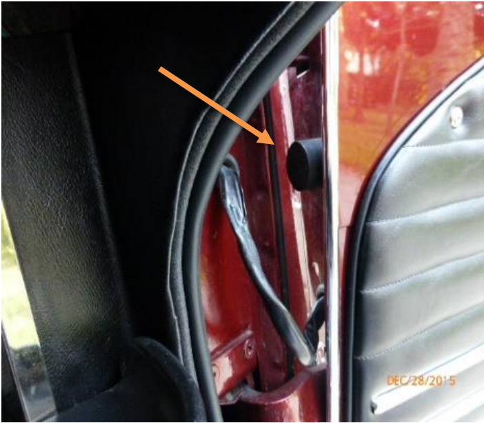
Rubber bumper which presses on door pillar Interior light switch
