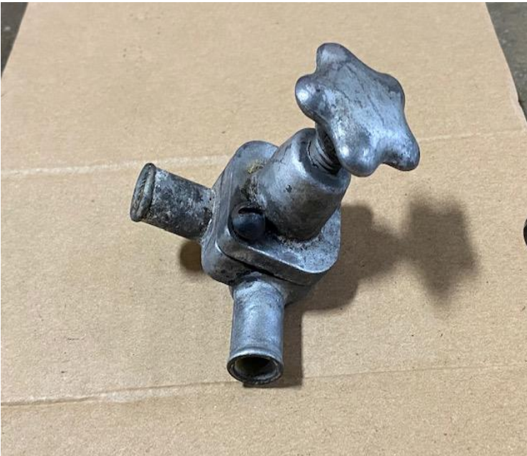
Manual heater cutoff valve
