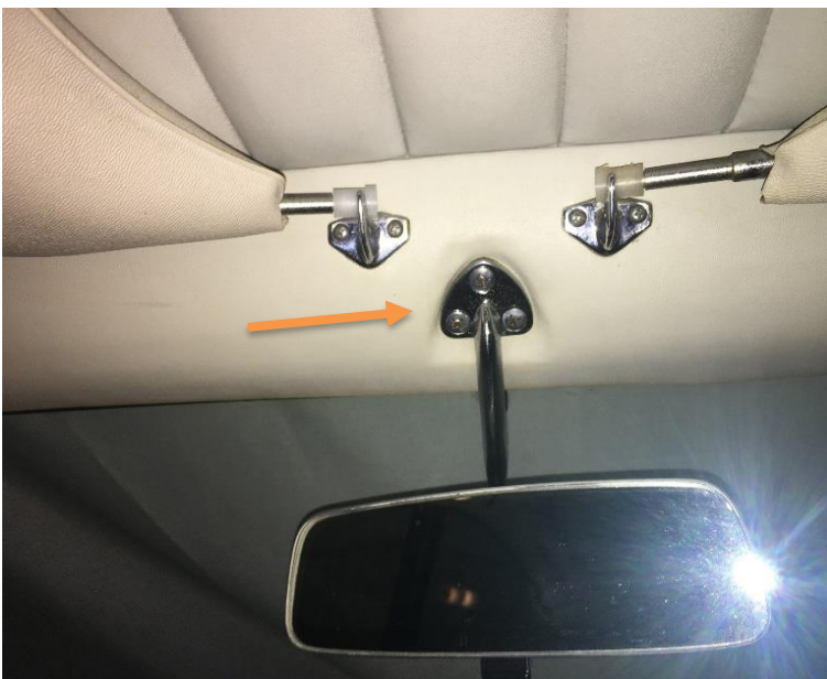
The mirror was mounted on the fabric in early cars as seen in car 8833
