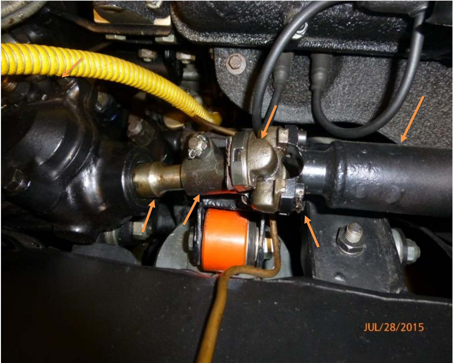
Steering box, coupler, U-joint, steering column
