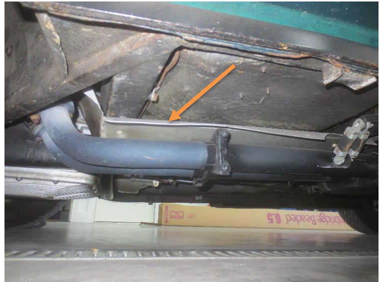
Heat shield over exhaust pipes in front of muffler, drivers side
