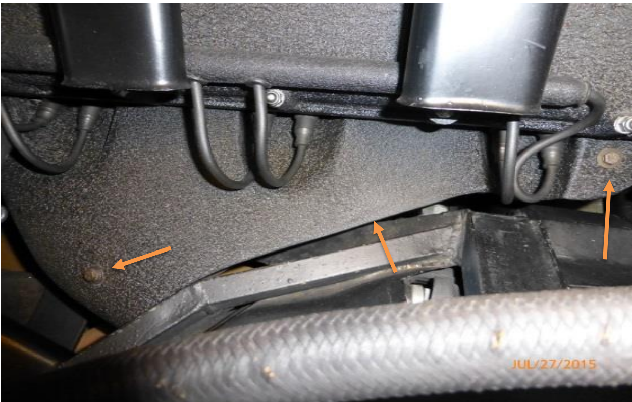
Heat shield, large washers, and Lobo bolts
