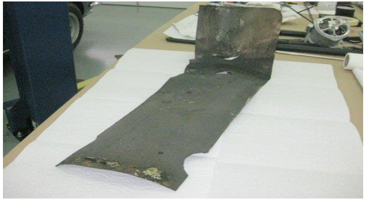
Heat shield over exhaust pipes on driver side
