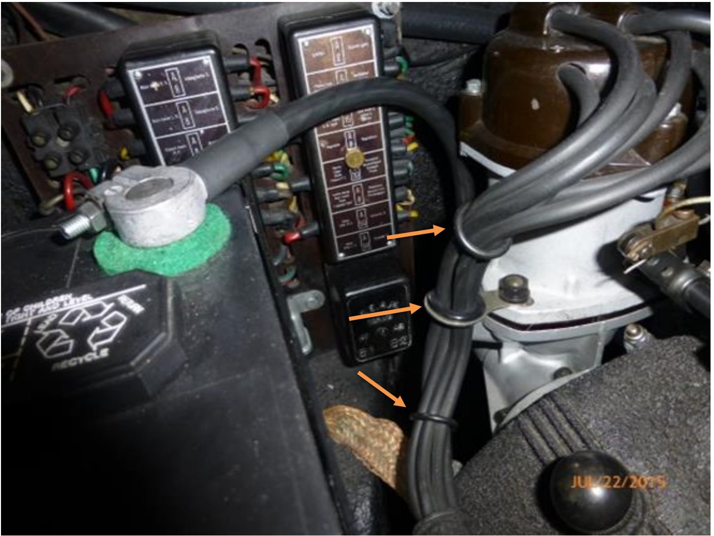
Retaining bracket on distributor and two O-rings gathering black 7mm plug wires , right side
