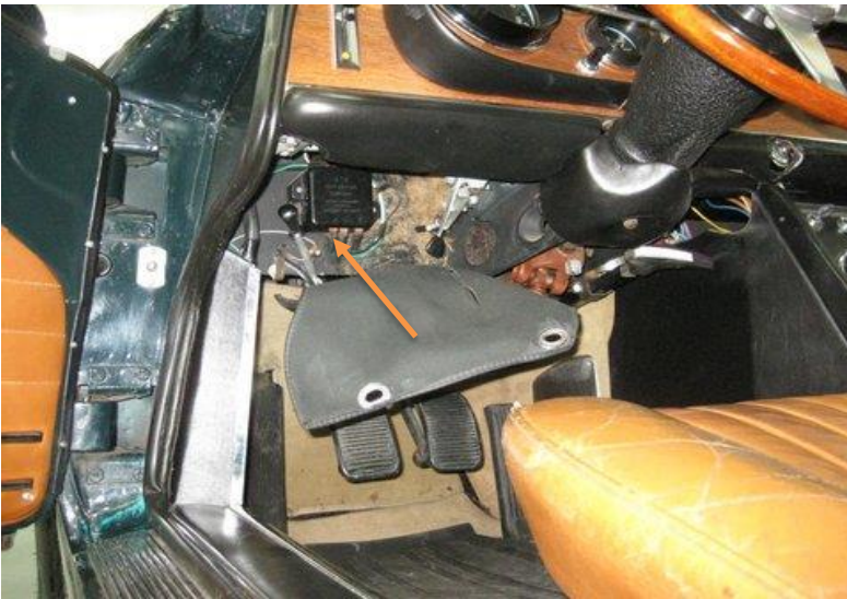
Lucas voltage regulator under dash
