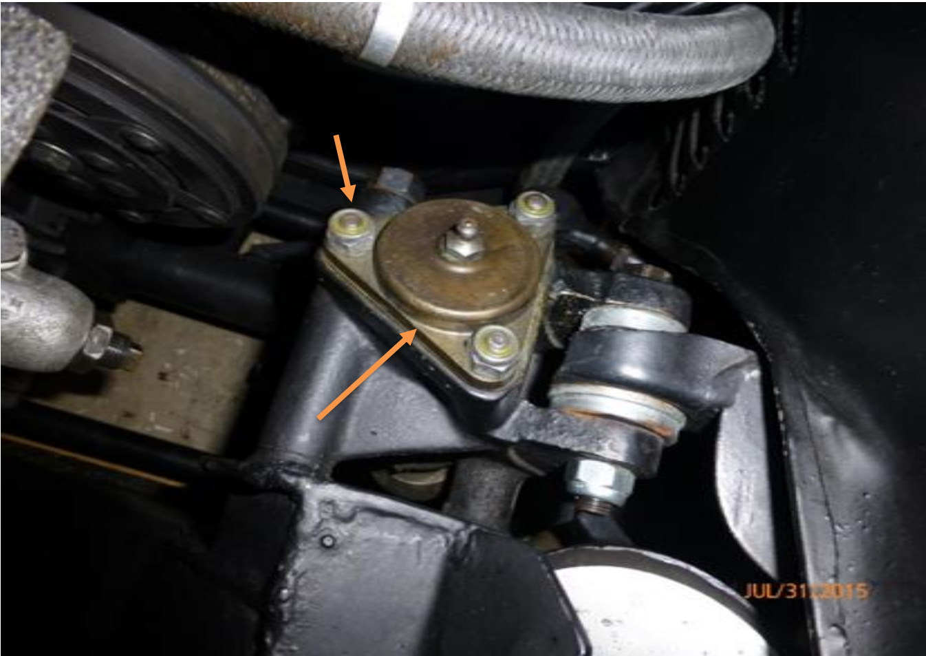
Steering Idler assembly, yellow insert on nuts
