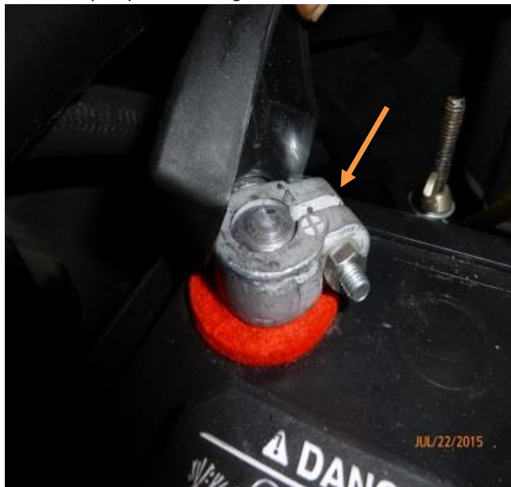
Positive terminal with rubber cap
