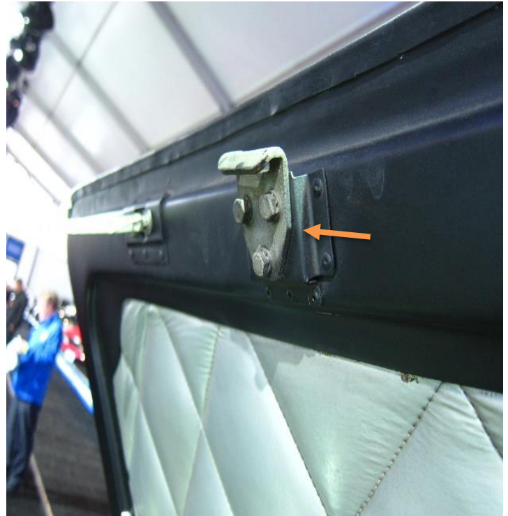
Unrestored car hood bracket with silver CAD bolts
