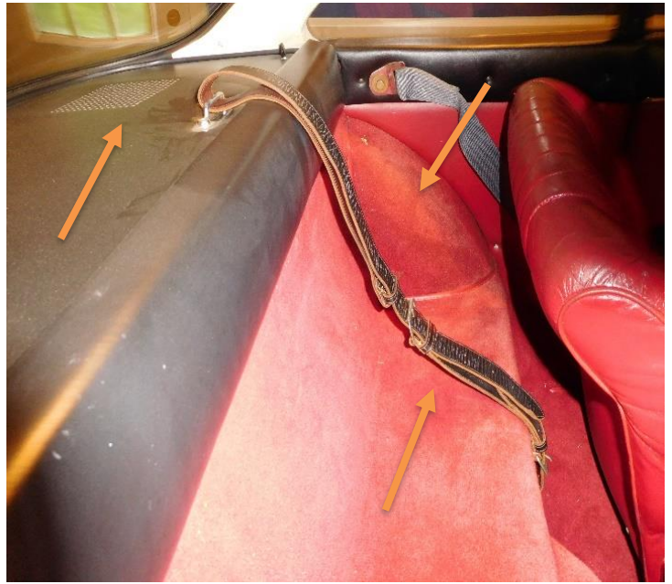
Unrestored car,10637, carpet covering wheelwell and speaker holes on rear parcel shelf, black and tan strap
