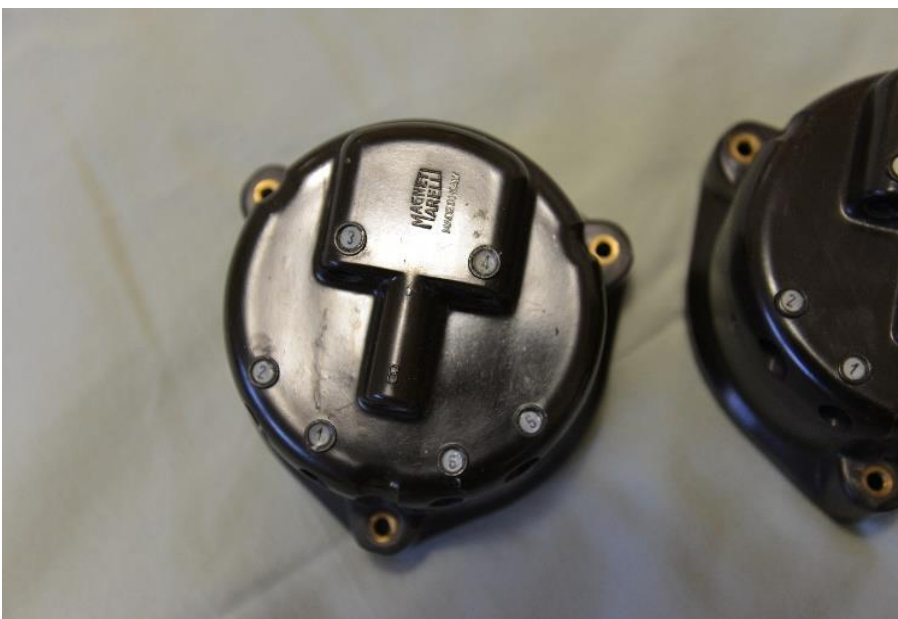
Distributor cap 1 thru 6 numbering on plug wire connections
