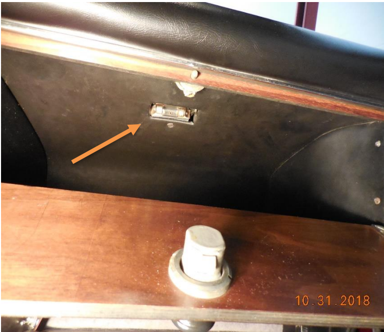
Light inside glove box with torpedo bulb
