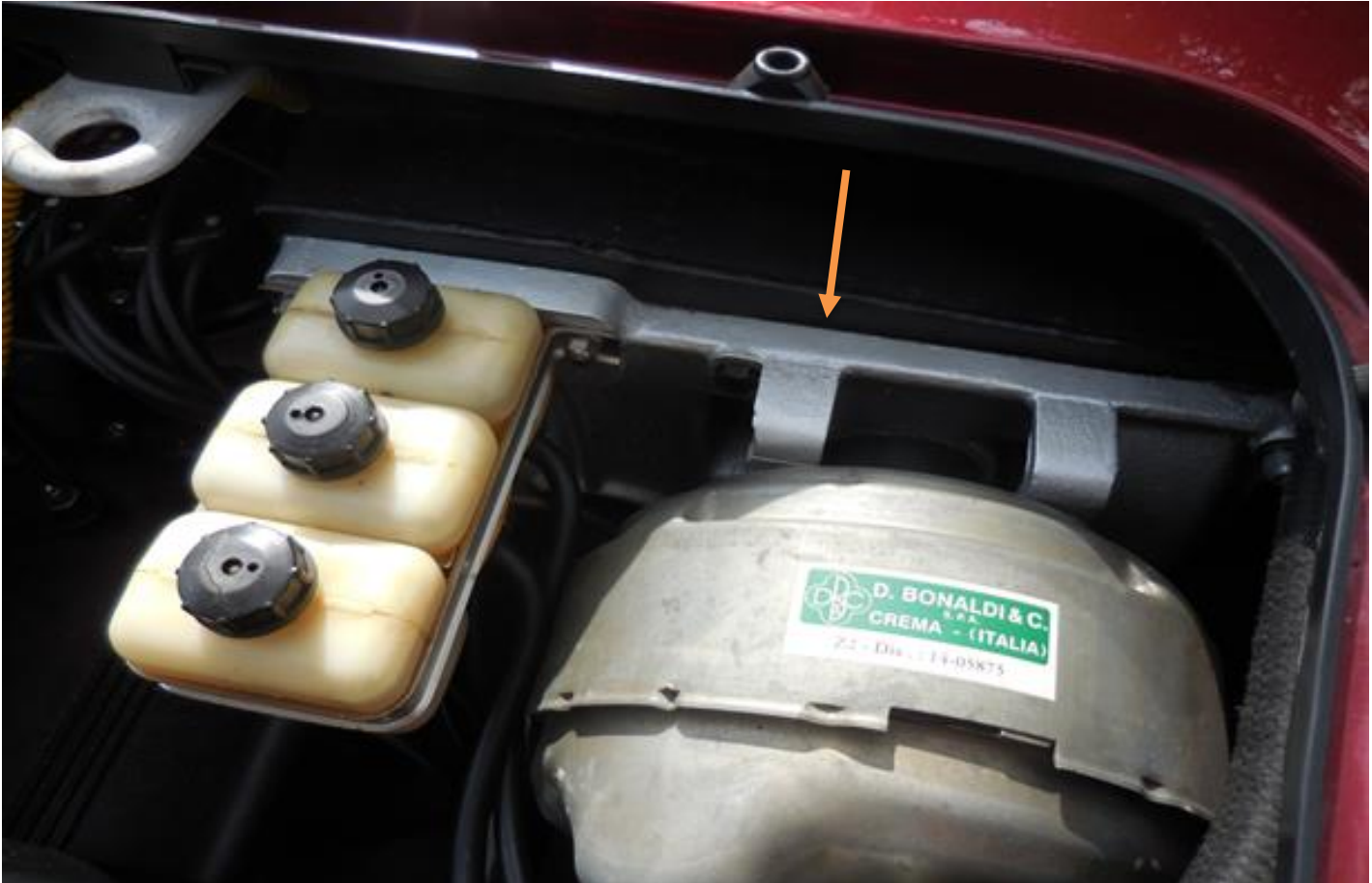
Cast base plate painted aluminum mounts the brake booster and fluid reservoirs
