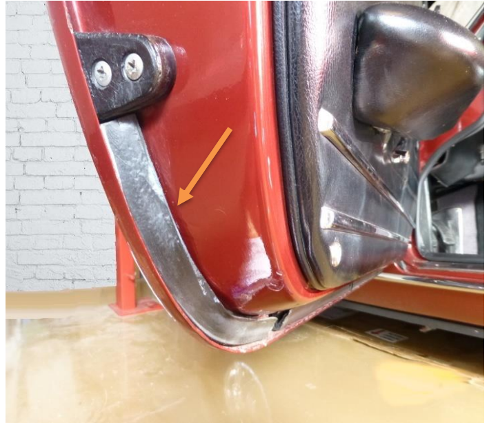
Rubber weather seal on bottom of door
