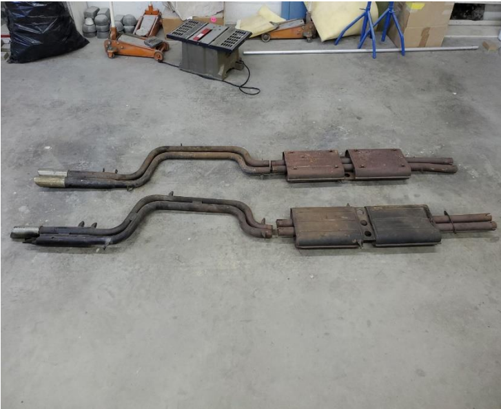
Original 330 GTC Ceretto exhaust system
