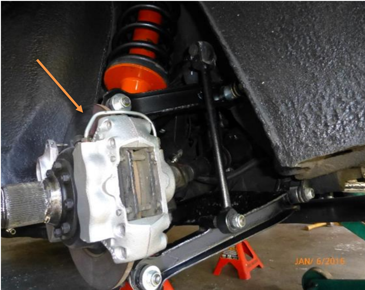
Rear suspension, silver CAD brake calipers
