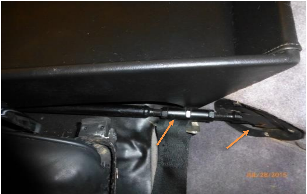
Shift rod from shift lever to the rear transaxle
